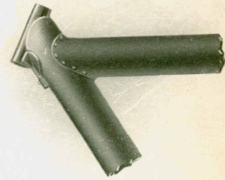
FRAME SHOWING RIVETS BEFORE FILING
